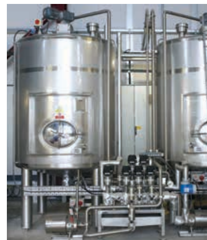
Yeast storage tank at the John Fergus & Co.'s new InchDairnie Distillery in Scotland
